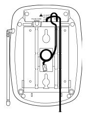
6. Plug the short modular cord into the wall plate jack, press the excess cord into the slot in the center of the bracket, then align the bracket's keyhole slots with the wall plate studs and slide the base downward to secure it.
